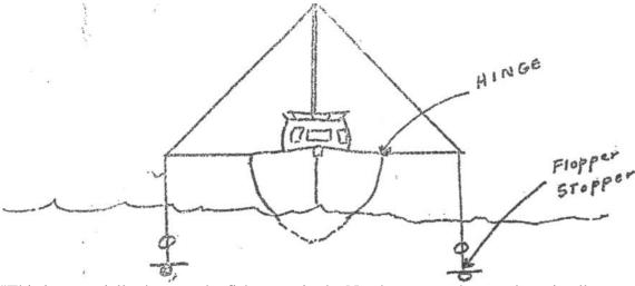
"This is essentially the way the fishermen in the Northwest use them and run in all kinds of weather. The simplest way, and the way I rigged it on the Vega, was to suspend the "flopper Stopper" from the end of the boom which was swung as far outboard as possible – about six feet – and secured there. Even this simple method I found quite effective in lessening the roll of the boat. It was particularly appreciated by guests with sensitive stomachs." (Ah so-o.)
